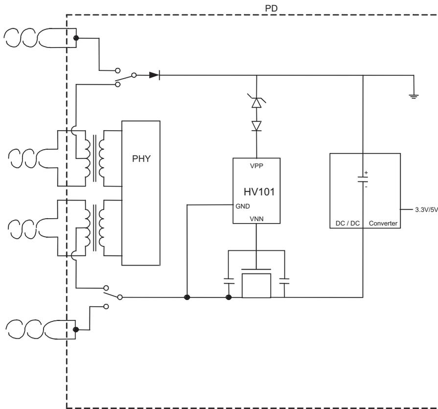
**HV101 Used as a UVLO & Load Switch**
