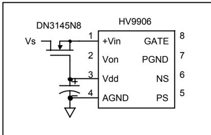
This method limits the +V<sub>IN</sub> voltage to V<sub>DD</sub> + V<sub>GS(OFF)</sub> of the depletion MOSFET for all input voltages and in fact raises the maximum allowable peak input voltage to the breakdown voltage rating of the depletion MOSFET. The worst-case power dissipation in the HV9906 is now given by the equation
