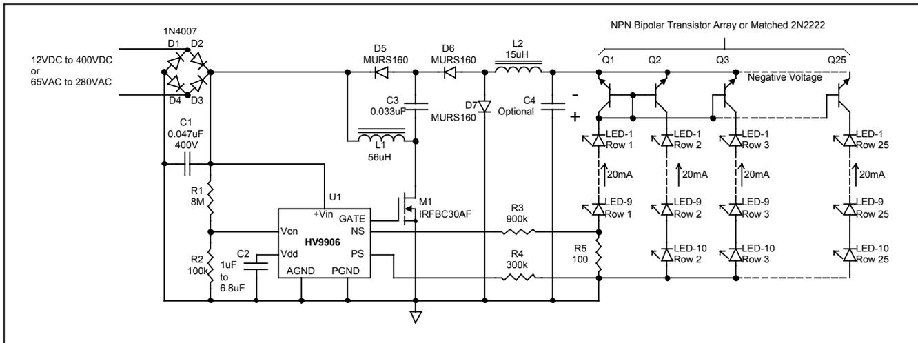
This circuit provides 0.5A constant average current output to power 249 LEDs, each operating at 20mA to form a large LED lamp or array. The circuit maintains a constant average current and the value of C4 capacitor controls the peak-to-peak ripple, which decreases with increasing capacitor value.
