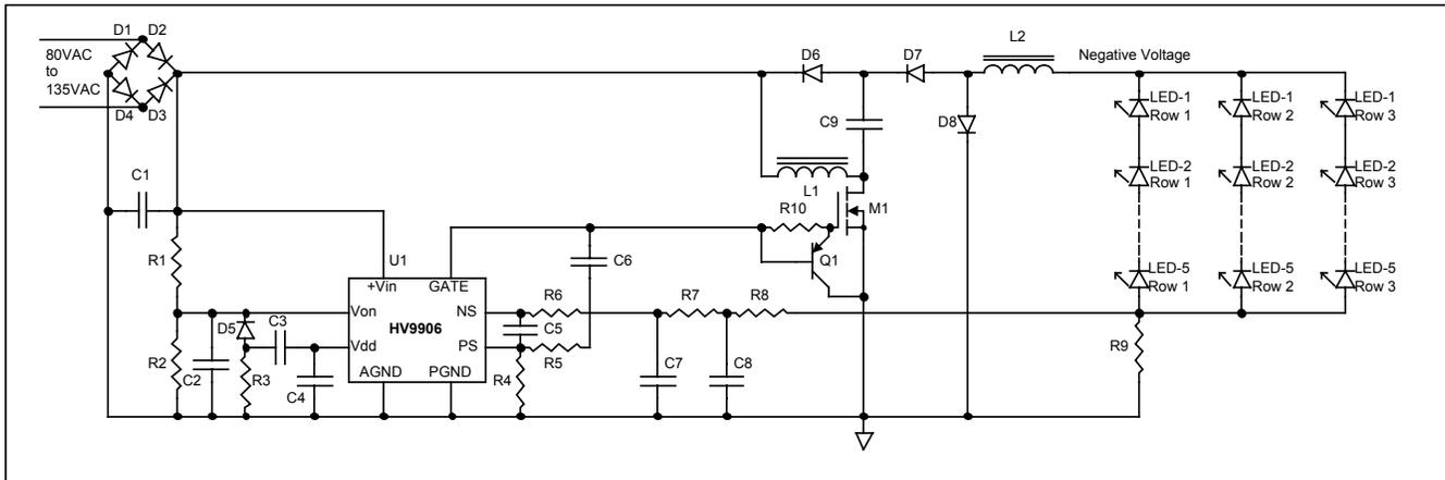
This power factor corrected circuit provides a constant average current output to power LED lamps.
