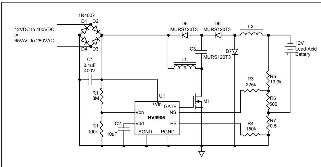
This floating battery charger circuit will charge a 6 cell 12V lead-acid battery to a float voltage of 13.8V and provides a 1A charging current limit for a severely discharged or shorted battery.
