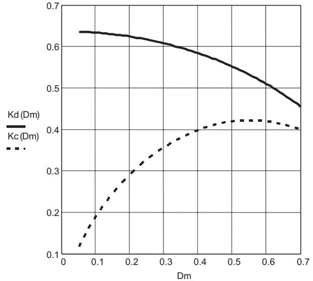
Fig. 1. Conduction Loss Coefficients  $K_C$  and  $K_d$
